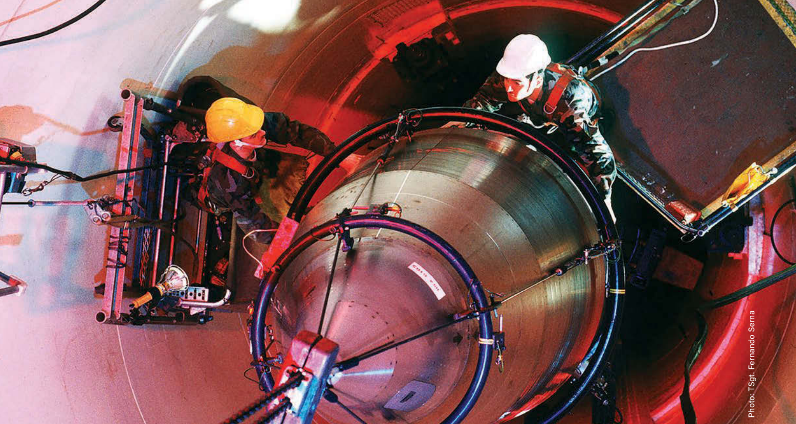
SrA. Scott Fowler (r) and SrA. Paul Gallegos (l) move the re-entry system of an LGM-30 Minuteman III missile onto a guidance set. The missiles are almost 50 years old.
